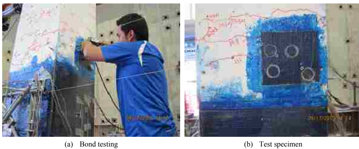
Figure B.2. Bond strength test
